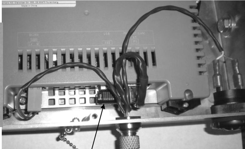
Each monitor touch screen has a USB memory card installed on the lower back side of the screen.
