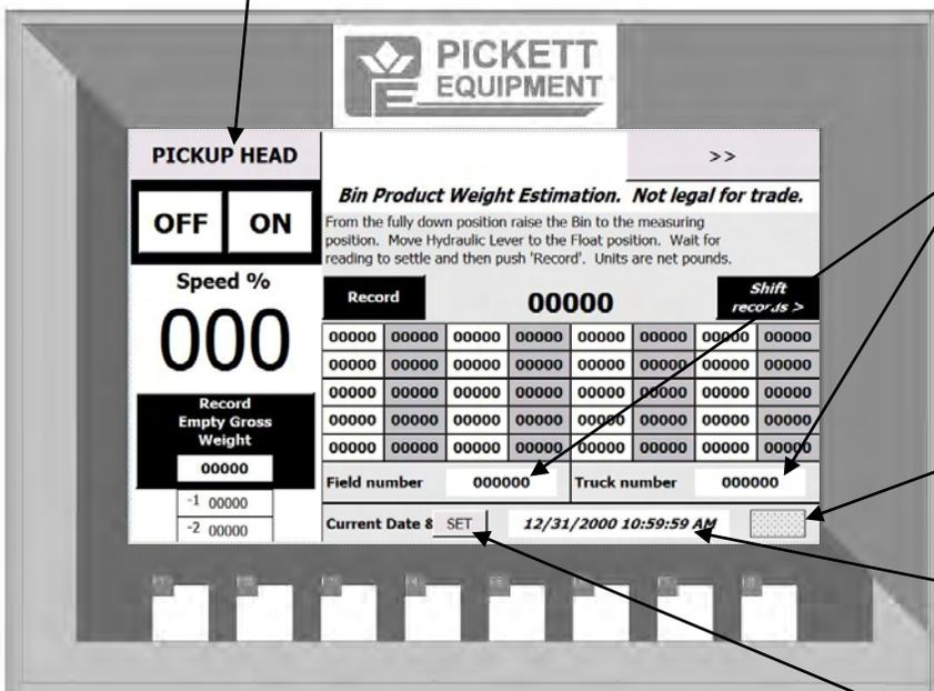
Field and truck numbers can be added touching the number area and typing in a number.
